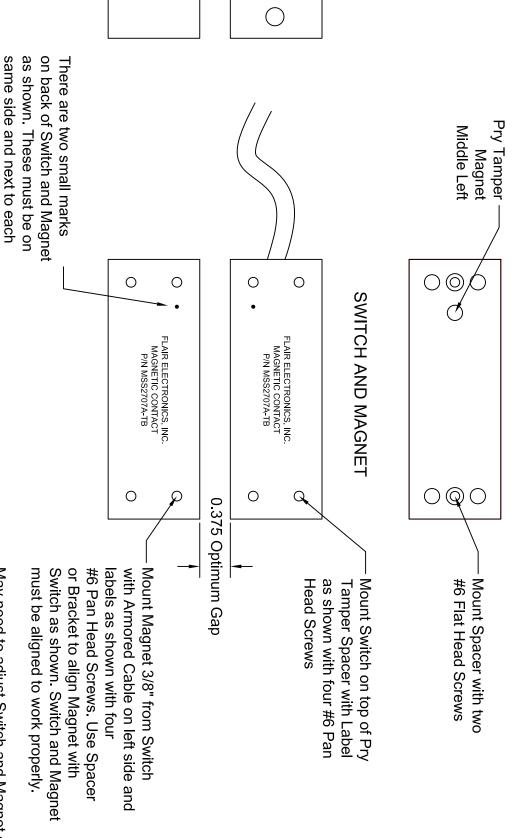
May need to adjust Switch and Magnet gap depending on material on which mounted.
